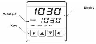
**Figure 2** – Front panel identification
