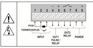
Figure 1 – Back panel connections
