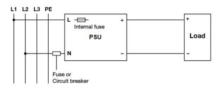
Fig. 4 2 of 3 Phase System Input Operation Connection Diagram
